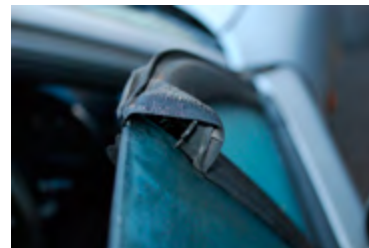
Drivers door window seal needed fettling
