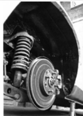
New coating of underseal for rear arches
